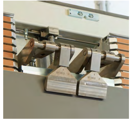
/ The clamping fixtures on the PAV panel lowering device ensure a secure grip and vertical transport.
