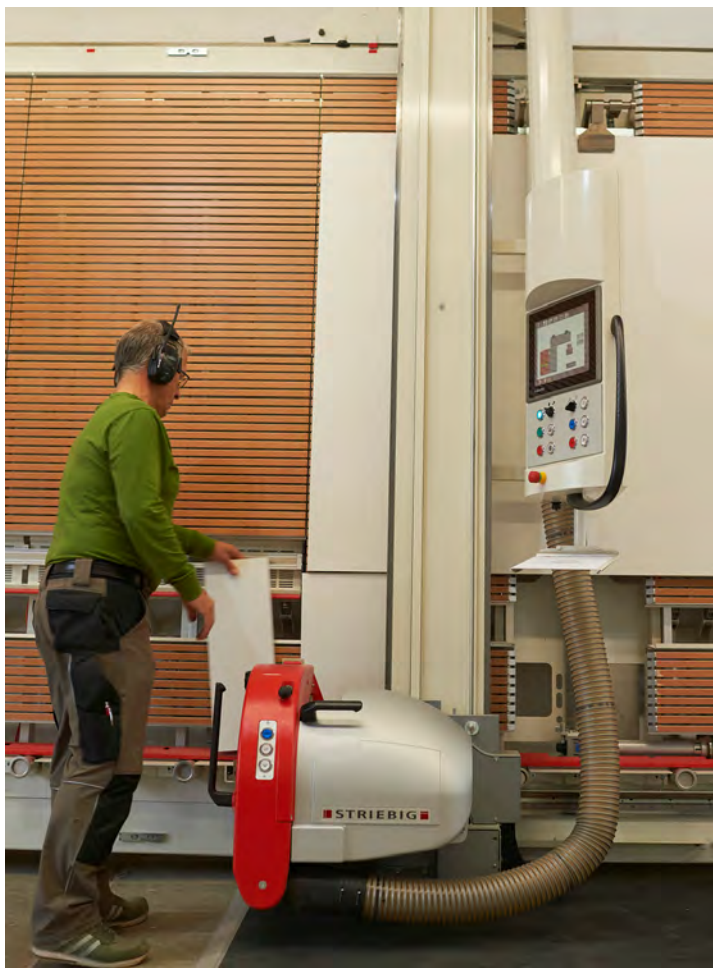
/ Panel cutting with the 4D is programmed and then carried out automatically. The workpiece just has to be manually picked up and labelled.
