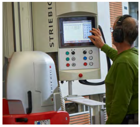
/ Place the panel on the panel saw, choose the programme using the touchscreen and start. Done.
