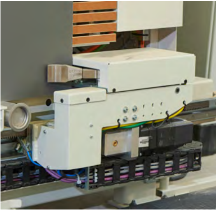
/ Automatic horizontal workpiece transport by means of the clamps on the programmable panel feeder.
