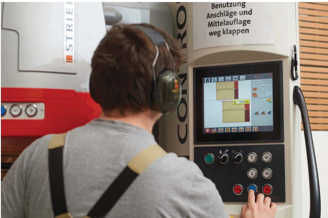
Fig. 1: CONTROL processes the cutting plan almost automatically. Pascal Klehr only removes the cut panel parts.
