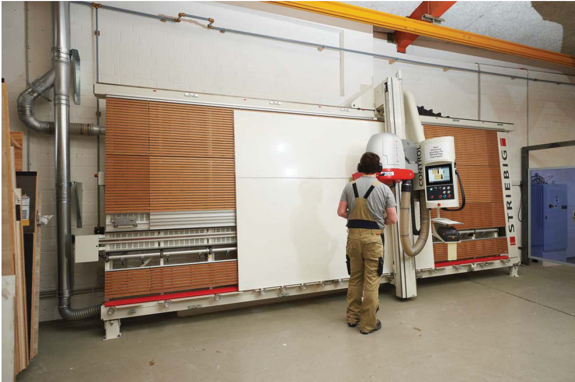
Fig. 1: CONTROL processes the cutting plan almost automatically. Pascal Klehr only removes the cut panel parts.
