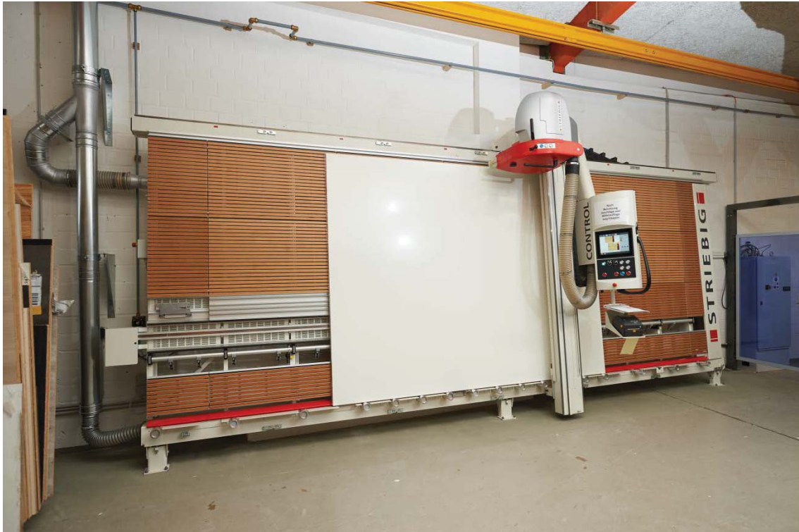
Fig. 6: One for almost everything: CONTROL with the ExpertCut CON option. 12" operating terminal, EPS.x electronic positioning system, ASP automatic saw beam positioning, label printer mounted directly under the operating terminal, LAN connection and cutting optimisation software ensure comfort and economy when cutting panels.
