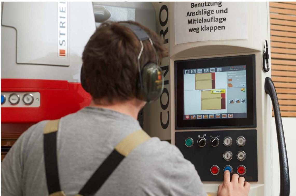
**Fig. 2: Clear cut plan display on the 12" touch screen.**
